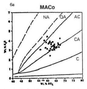
Figure 2. Alkali-calcic, oxidized plutons: whole rock chemistry of igneous rocks associated with lead-zinc-silver deposits (Wilt, 1995)
