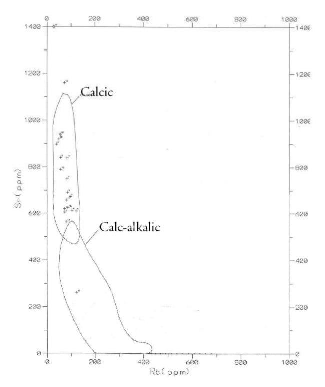
Figure 22. Rubidium vs. strontium plot showing fields of peraluminous calcic and calc-alkalic, oxidized plutons indicating whole rock chemistry of igneous rocks associated with gold (calcic) or tungsten (calc-alkalic) deposits (Keith and others, 1995)
