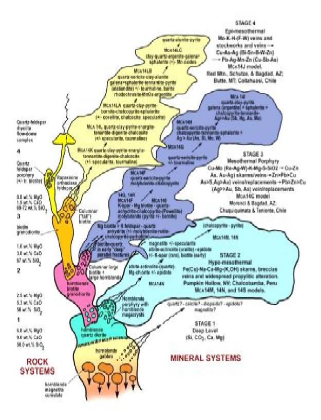
Figure 20. Stages of fluid release and differentiation products of calc-alkalic, oxidized plutons (Keith)
